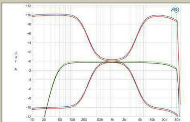
Fig.10 Harman Kardon HK 990, balanced input, DSP On, Subwoofer Off, frequency response at 2.83V into 8 ohms with Treble and Bass controls at \pm 10 dB (left channel blue, right red), and with tone controls at 0dB but Subwoofer On (left green, right gray). (2dB/vertical div.)
