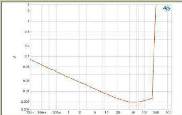
Fig.12 Harman Kardon HK 990, Direct Path, distortion (%) vs 1kHz continuous output power into 8 ohms.
